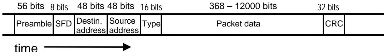
Within the “Packet data” are additional layers of more protocols, for the case of computer networking. Embedded within that is the actual user data.
